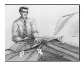
4. Attach the two snaps on the inside flap of the side cover to the top of the quarter trim panel. Attach the front snap (E) first and then the rear snap (F). The rear snap is adjustable for ease of installation.
